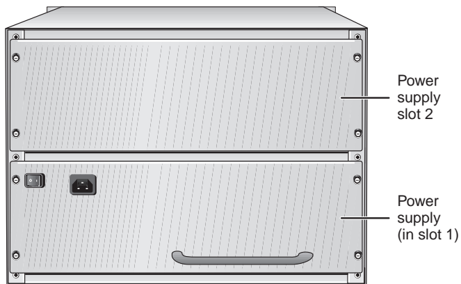
Figure 3 930-watt AC Power Supply in the Switch 4007
